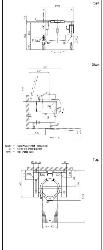
ProThermetic Sprint Electric Tilting Boiling Pan, 60lt Hygienic Profile, Freestanding
